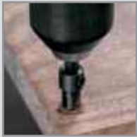
COUNTERSINK Pre-drills hole for the fastener and prevents the workpiece from splitting
