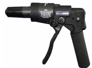
D-700C Riveter-Nutsetter Pull Force: 5,000 lbs. Stroke: 0.800"
