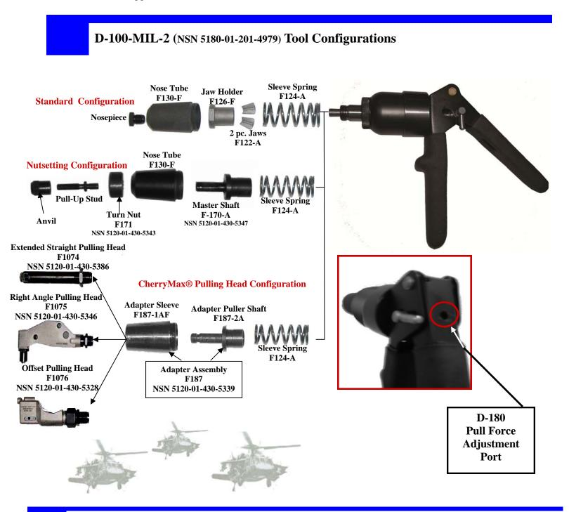
**NOTE:** The CherryMax® Offset, Right Angle, and Extended Straight Pulling Heads, included in the D-100-MIL-2 are not a part of the D-100-MIL-1 kit; however space is provided so that they may be added as needed. The kits are supplied in a weather tight metal carrying case (2 1/2" x 6 1/2" x 10") along with operating instructions, parts list and warranty card.
