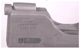
Adjustment should provide resistance to be felt when inserting the 5/32" and 3/16" stems into the pulling head
