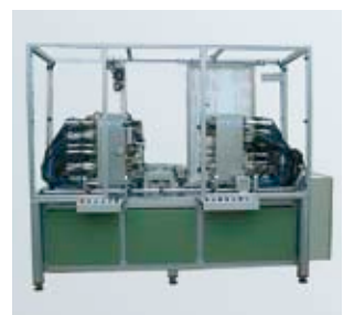
23 placing heads to assemble a computer chassis
