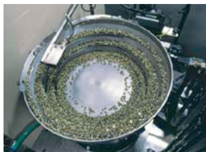
Fasteners fed via a vibrating bowl
