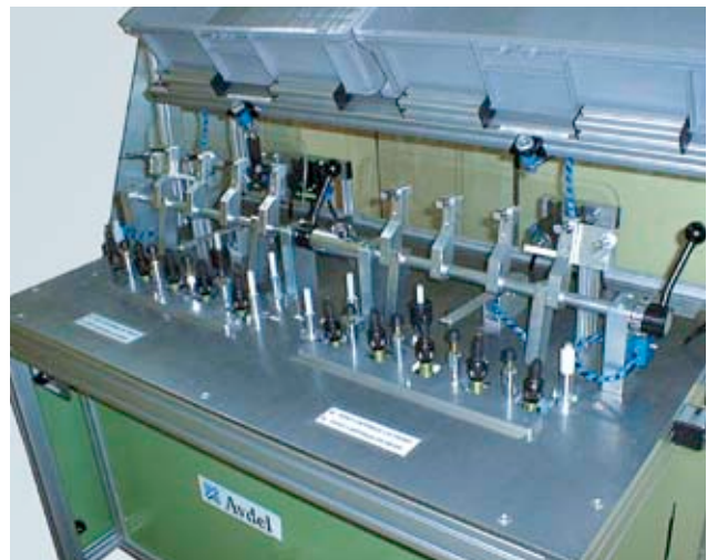
10 placing heads to assemble automotive sealing strips
