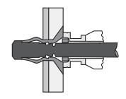
The continued pulling action compresses the large bulb bearing area against the backside of the structure.
