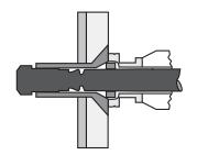
The pulling action on the stem causes the sleeve to start bulbing away from the backside of the structure, thereby eliminating exit hole delamination.
