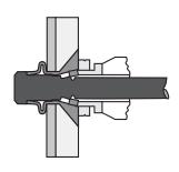
The stem is fractured at the break notch by continued pulling on the stem, thereby providing a flush, burr-free, installation.
